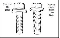
Note: DO NOT reuse the bolts removed from the TRD calipers. They are a different thread pitch than the OE caliper. **NEW** bolts must be used.
