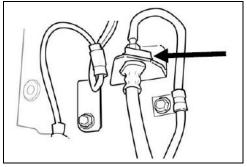
c. Install the **NEW** brake hose retaining clip.
