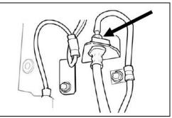
e. Using a flare nut wrench, separate the steel line union from the brake hose.
