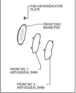
b. Install the **NEW** anti-squeal shims to the **NEW** disc brake pads.
