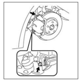
e. Install the **NEW** disc brake cylinder assembly into place and install the 2 bolts.
