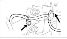
d. Remove the 2 bolts securing the hose to the steering knuckle and strut.
