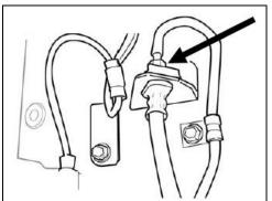
d. Using a flare nut wrench, install the steel line union to the flexible brake hose.
