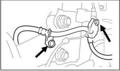
b. Install the 2 bolts securing the **NEW** flexible hose to the steering knuckle and strut.
