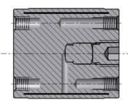
ETP-EXPAND, a very compact design without flange and the pressure setting mechanism integrated in the center. Used for frequent and quick positioning of a hub in the health care industry.
