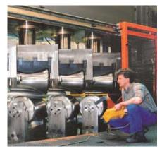
Machine for cold forming of steel tubes. ETP-OCTOPUS locks the pistons of hydraulic cylinders, one for each cylinder, in a certain position when forming different sizes of tubes. The position is changed rather often. The locking with ETP-OCTOPUS can be done all at the same time from a central located hydraulic pump. ETP-OCTOPUS is plated in the bore with aluminium bronze to reduce wear.
