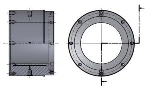
ETP-OCTOPUS with hydraulic connection on the outer diameter. The parts to fix and move are locked with a screw joint to the ends of ETP-OCTOPUS. One hydraulic connection on each side in order to reach one easily.
