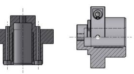
ETP product for accurate locking of a component in the machine tool industry. The component is accurately locked to the flange with screws then centered when tightening the screw.
