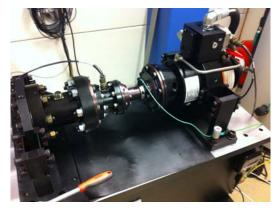
Fatigue torque test machine
