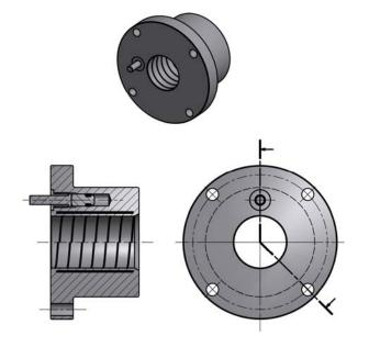
ETP-AXPRESS, for frequent and quick clamping a pin is moved to push the piston. A hydraulic cylinder is used to create the force on the pin. ETP-AXPRESS only clamps to the inside. Spiral tracks on the inner diameter makes the clamping surfaces less sensitive for impurities.
