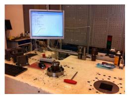
Slip torque test machine
