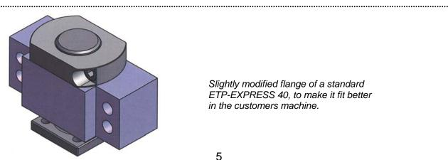
Slightly modified flange of a standard ETP-EXPRESS 40, to make it fit better in the customers machine.
