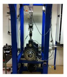
Radial loads and bending torque fatigue test machine
