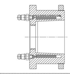
ETP-HYLOC only clamping to the inside. A component is locked with a nut onto the shoulder on the outside diameter.
