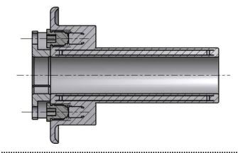
ETP product with fixed inner/outer diameter due to customers machine design. Safety locking ring included if pressurizing is forgotten – also works as a stop for the tightening screws. Flange for easy lifting and protection of the hub.
