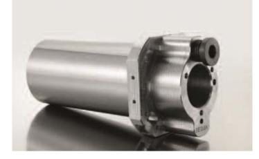
ETP-AXPRESS with the pressure screw in the axial direction. Is designed for fastening & centering of decoration roller for printing on the outside of beverage cans. The tightening is done with a screw with a flange. The flange makes sure the screw is not overtightened. The tightening has to be in the axial direction because of the design of the machine. All unnecessary material is machined away on the flange part to reduce weight.
