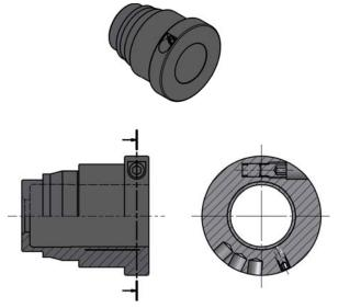
ETP-EXPRESS only clamping to the inside. On the outside different components are fixed.
