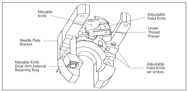
Figure 4 - 12 Underside View of Trimmer Parts
