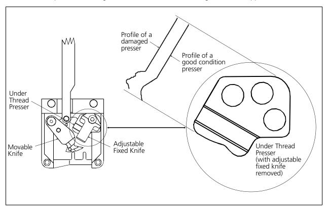
Figure 4 - 9 Under Thread Presser
