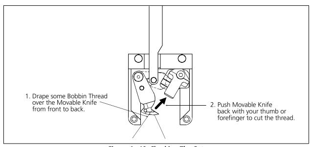
Figure 4 - 10 Checking The Cut
