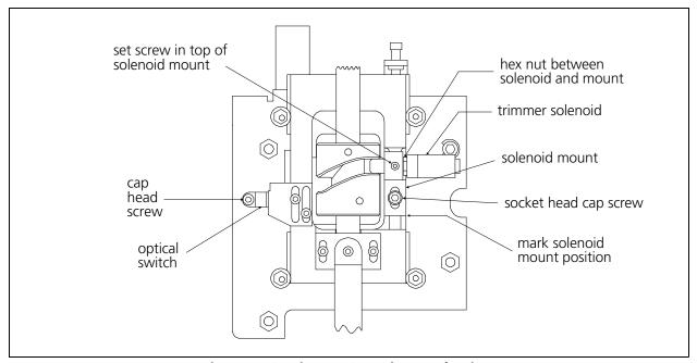
Figure 4 - 3 Trimmer Camming Mechanism
