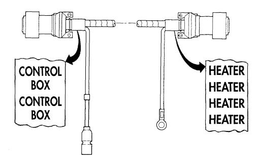
g. The decals shown below are located on the radiator and are common to all M939/A1/A2 series vehicles.
