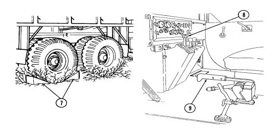
(2) Place transmission selector lever (8) in 1-5 (drive) and transfer case shift lever (9) in low range. Slowly accelerate without causing wheels to spin or engine to race. Place transfer case shift lever (9) in high range when under way.
