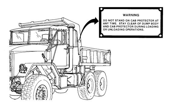
The plate shown below is located on the hard top installed on M939/A1/A2 series vehicles.
