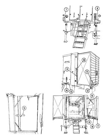
(16) Turn ratchet wrench (8) clockwise to lock floor (5) and roof (1) panels in position.
