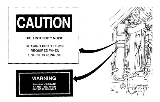
h. The decal shown below is located on the surge tank and is common to all M939/A1/A2 series vehicles.
