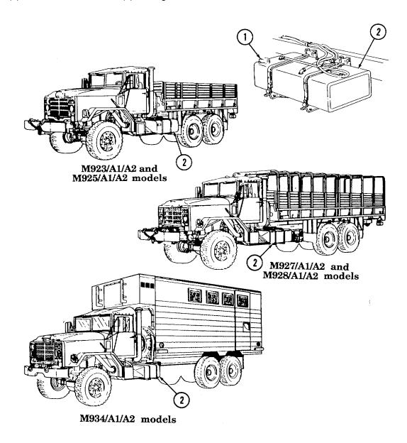
(b) Location of fuel tanks (2) on dual tank model vehicles:
