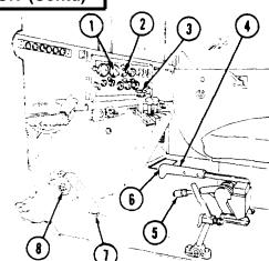
$j_{\perp}$  Shift transfer case shift lever (4) as required by vehicle speed and changes in driving conditions.
