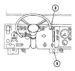
(6) Press in trailer air supply valve control knob (9) and hold in place for 15 seconds. Release valve control knob (9). Valve control knob (9) should remain in pressed-in position indicating trailer or artillery load airbrake system has proper air pressure.
