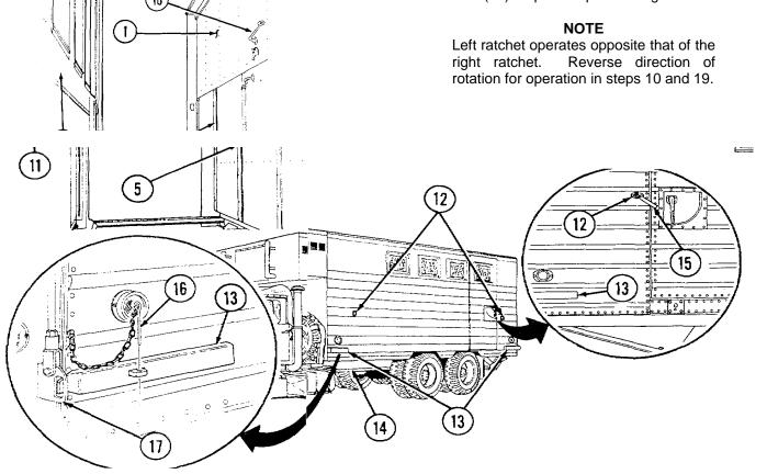
(21) Turn four side locks (12) clockwise with side panel lockwrench (15) and insert all four corner ends of lock handle assembly (13) into retaining bracket (17). Close lock handle assembly (13) and secure in place with chained pin (16).
