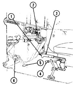
h. Release brake pedal (6) and depress accelerator pedal (5). Accelerate at a safe, steady speed.
