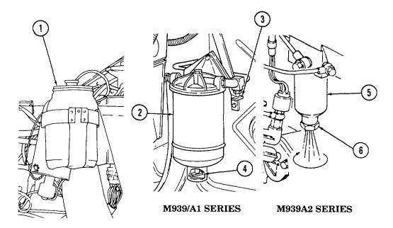
(a) On M939/A1 series vehicles, open fuel drainvalves (3) and (4) on fuel filter/water separator (2) and drain water into suitable container. Close drainvalves (3) and (4) when clear fuel is visible.
