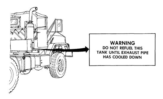
j. The caution plates shown below are common only to the dropside cargo (M923/A1/A2, M925/A1/A2) model vehicles.
