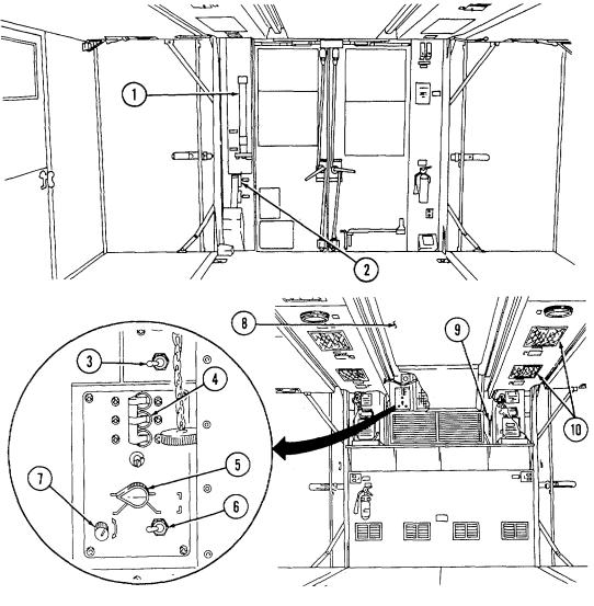
(7) Adjust temperature selector (7). Cooler temperatures are obtained when temperature selector (7) is turned counterclockwise.
