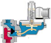
which there is no-flow and the regulator is closed is defined as lock-up.
