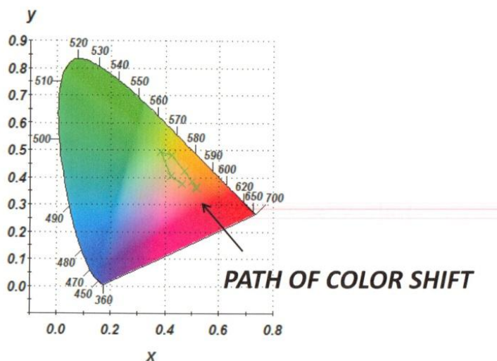
Figure 17. Shift in reflectance of Ag/SiO 2 /Ag Fabry Perot filter.
