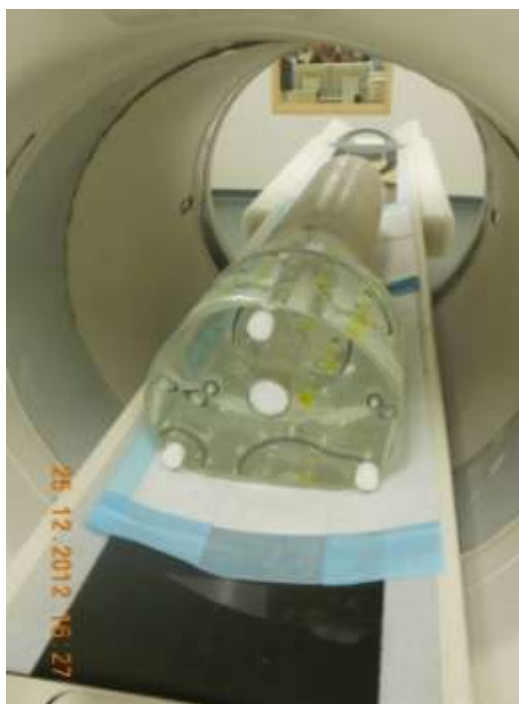
Figure 15: IEC body Phantom and 70 cm plastic cylinder (scatter phantom) set up during the test.
