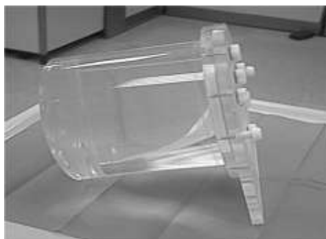
Figure 23: A cylinder phantom to be filled with ^{18}\text{F} solution. Phantoms like this are used for normalization of the PET detector, for radioactivity concentration calibration and for uniformity testing.
