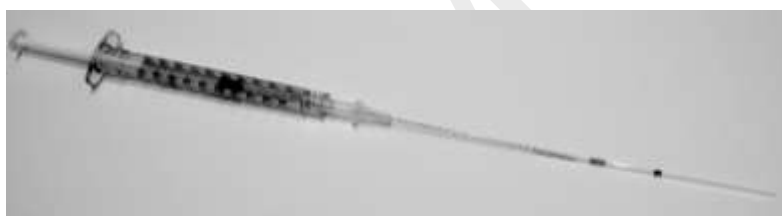
Figure 4: A syringe of the type with a fine needle to put a small amount of ^{18}\text{F} solution inside a capillary tube (on right) for the measurement of spatial resolution
