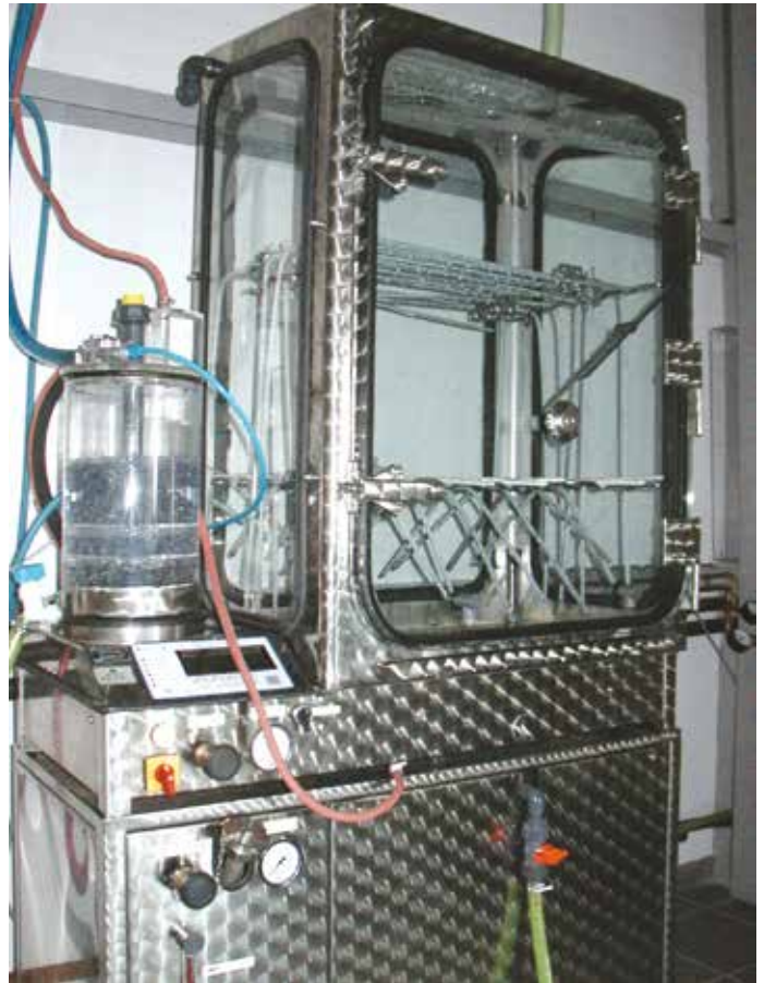
Environmental ageing chamber for ammonia atmosphere ageing
