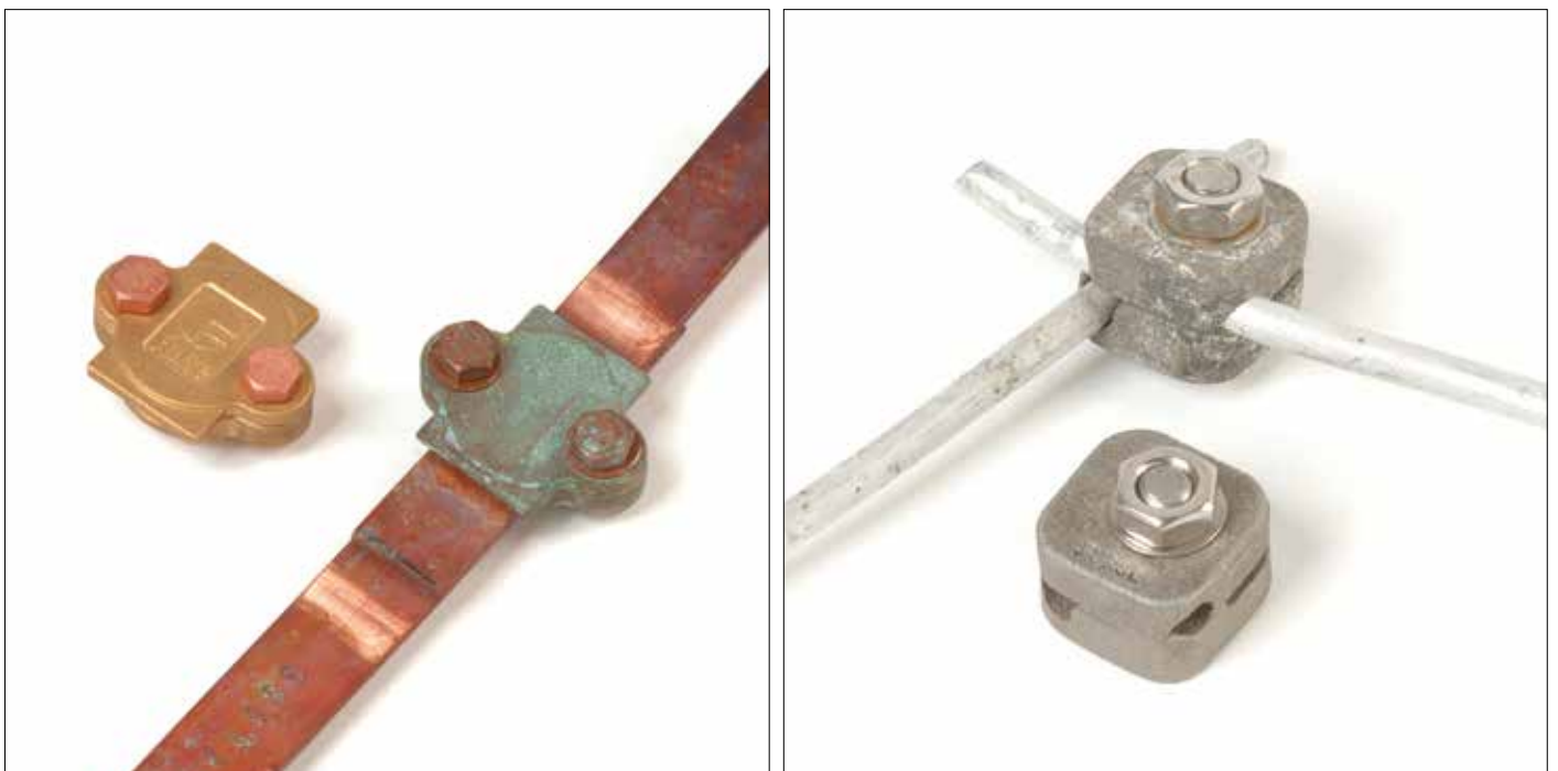
Figure 14. Furse lightning protection components, showing results after environmental preconditioning and lightning discharge testing
