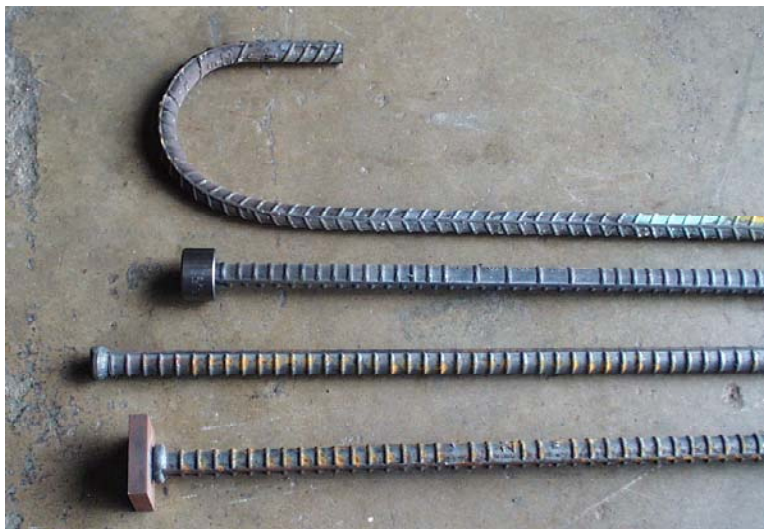
Figure 1.1: Various headed bars compared to a standard hook (#8 size)
