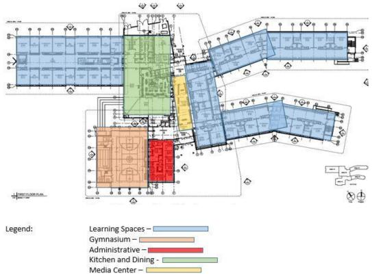
Figure 1: First Floor Plan with Basic Programming
