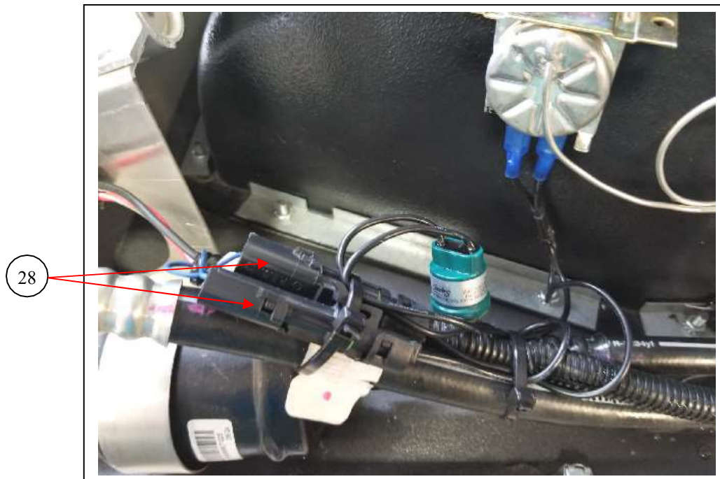
28. Plug thermostat wiring into wire harness, secure wiring and connectors to hoses with 02 000 052 wire ties.
