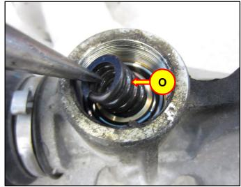
15. Clean the threads and interior of yoke plug housing with a clean rag and isopropyl alcohol.
