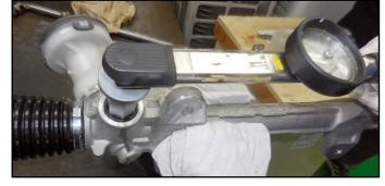
24a. Set the final torque of the yoke plug:
