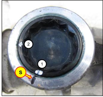
b. Rotate the yoke plug <u>counter-clockwise</u> until the white yoke plug mark labeled (2) reaches the steering rack housing mark labeled (S).
