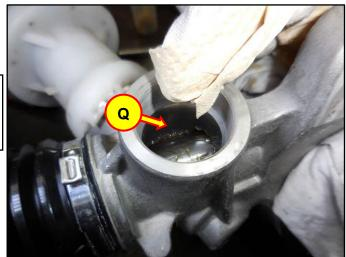
19. Apply the grease evenly on the contact side of the new rack bar support yoke.
