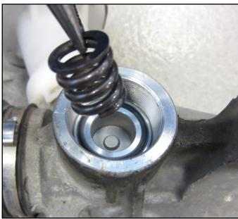
22. Hand tighten the new yoke plug.
