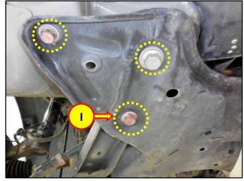
9. Carefully lower the sub frame to provide access to the steering rack (J).
