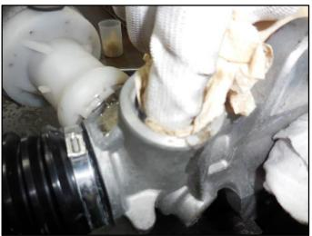
16. Clean out the remaining debris with an air gun.
