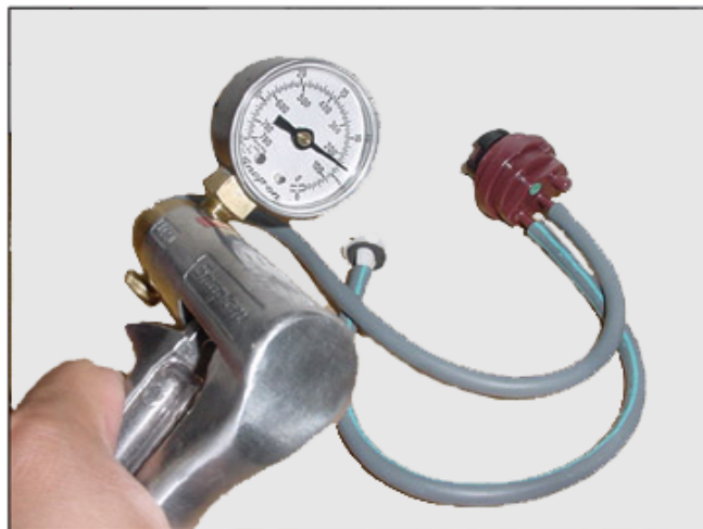
The Vacuum Control Valve is Regulating Vacuum to 7in-Hg.
