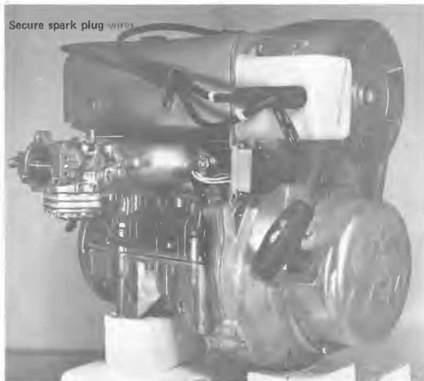
Fig. 5-12 Recoil Starter Installed
