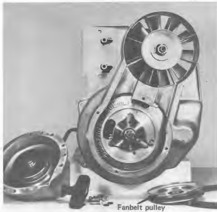
Fig. 3-4 Starter cup and fan belt pulley removed.
