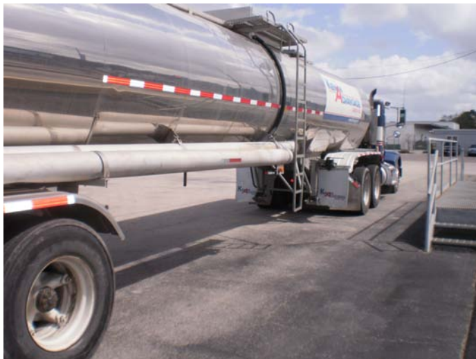
MC 407 Trailer- no bottom fittings in center of trailer.
