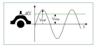
Figure 12. Bearing velocity (Vrms): RMS.
