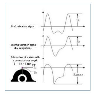
Figure 9. Absolute shaft vibration Sp-p:. Peak to Peak Displacement.
