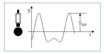
Figure 25. Analysis of the shaft eccentricity of min/max.
