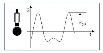
Figure 3. Shaft vibration So-p: 0 to Peak Displacement.
