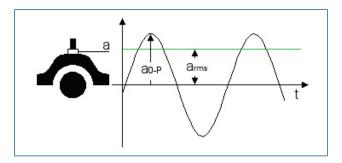
Figure 10. Bearing acceleration RMS (arms): RMS.
