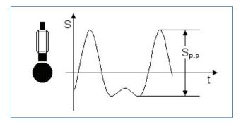
Figure 24. Analysis of the shaft eccentricity in peak-peak.
