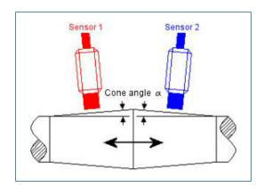
Figure 22. Double-cone measurement set up.
