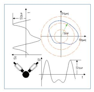
Figure 6. Shaft vibration So-p max: 0 to Peak
