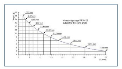
Figure 23. Axial measuring range versus cone angle.
