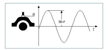
Figure 11. Bearing acceleration Peak (ao-p): 0 to Peak.
