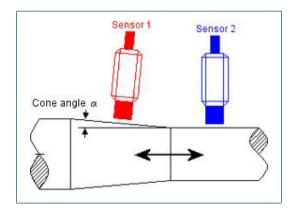
Figure 21. Single-cone measurement set up.
