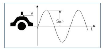
Figure 14. Bearing vibration So-p: 0 to Peak.
