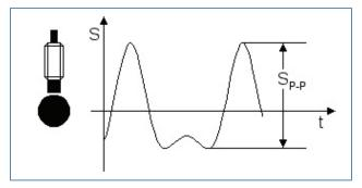
Figure 4. Shaft vibration Sp-p: Peak to Peak Displacement.
