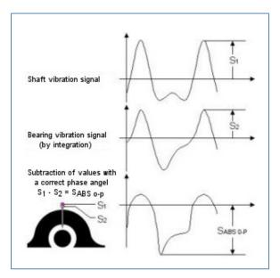
Figure 8. Absolute shaft vibration So-p: 0 to Peak Displacement.
