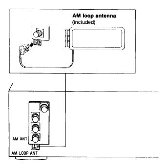
Connect the AM loop antenna to the AM loop antenna terminals, and mount it vertically to the rear panel of this unit.
