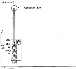
Attach to a wall (using a tape) facing in the direction of best reception.
