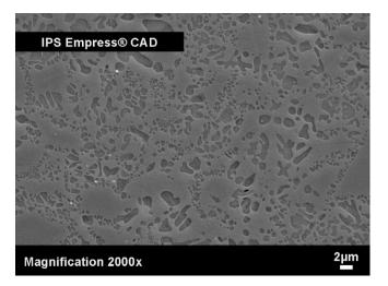
SEM of IPS Empress<sup>®</sup> CAD milling block with a leucite crystal content of 35 to 45 vol % with crystalline size of 1-5  $\mu$ m.
