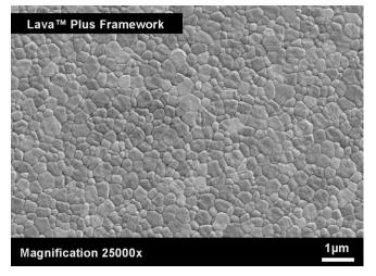
SEM of the new more translucent Lava<sup>™</sup> Plus ZrO<sub>2</sub> (about 0.3 μm particle size).
