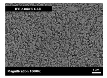
SEM of IPS e.max<sup>®</sup> CAD lithium disilicate. The high crystalline content (~70%) incorporated in a glass matrix produces a high strength ceramic without compromising translucency.
