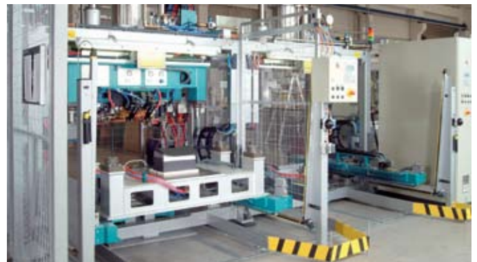
Sliding table double press laminating unit (pneumatic) with fast tool change
