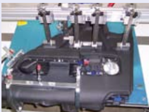
Component on positioning fixtures
