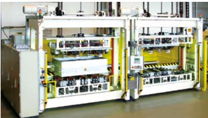
Double press laminating unit (electric motor driven)
