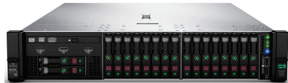
HPE ProLiant DL560 Gen10 (shown with box 1 populated with the Universal Media Bay and boxes 2 and 3 with 8 SFF drives)
