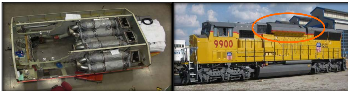
Figure V-1: UP 9900: DOC/DPF Aftertreatment System (left picture)(About 4.5 tons) (SMAQMD et al., 2012)
