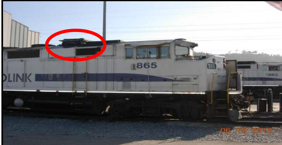
Figure V-4: An EF&EE Compact SCR and DOC System Retrofitted Onto a Metrolink Passenger Locomotive (EF&EE, 2010b)
