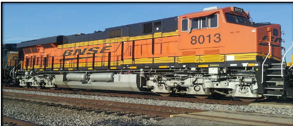
Figure I-4: Freight Interstate Line Haul Locomotive BNSF 8013 2014 Model Year – Tier 3 – (Up to 183,000 Pounds of Pulling Power) (RR Picture Archives, 2014a)
