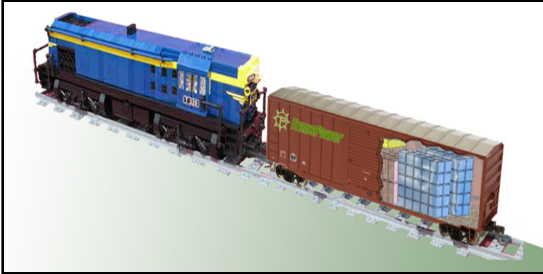
Figure VI-4: Transpower Concept for Battery Tender (Transpower, 2012)
