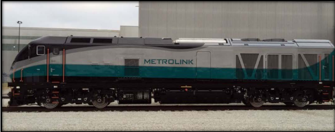
Figure I-6: New Metrolink EMD Tier 4 Passenger Locomotive Caterpillar High-Speed 4,700 hp Engine (Metrolink News, 2016)
