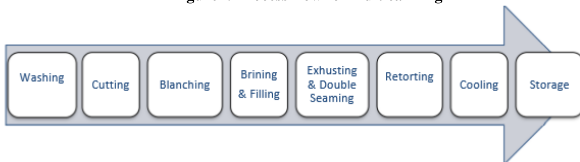
Figure3: Process flow for vegetable canning
