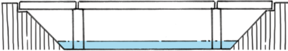
A: A beam and column bridge
