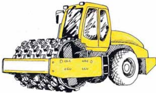
Figure 10: A road roller
