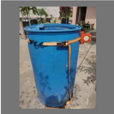
Pneumatic Ball Vibrator with Ratchet and Strap Arrangement from drum
