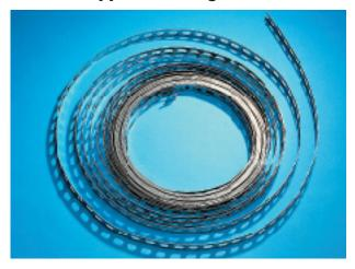
Manufactured from corrosion resistant galvanised mild steel strip 0.9mm thick, and supplied in 30 metre coils. The elongated holes are punched at 30mm pitch to simplify alignment and fixing. Complies with the requirements of DW144.
