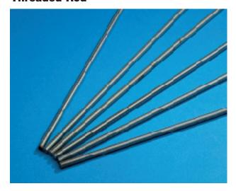
Threaded rod is manufactured from mild steel, zinc plated. Supplied in 3 metre lengths and available in M6, M8, M10 and M12 sizes. Studding connectors are also available to reduce wastage to a minimum.
