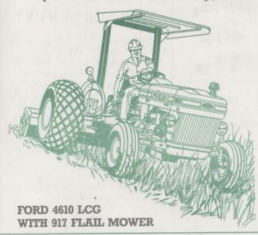
Ford LCG tractors are especially designed for mowing on slopes. With their wide-set axles and low center-of-gravity, they really hug the ground.
