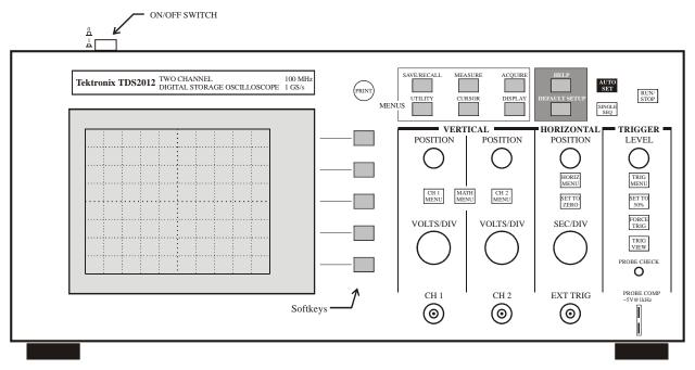
Figure 1 Front panel layout of TDS2012 Digital Storage Oscilloscope.
