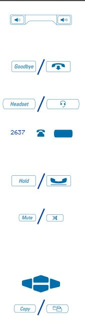
Use the **Volume Control Bar** to control the volume of the handset, headset, speaker, ringer, and handsfree. Increase the volume by pressing the right side of the bar. Lower it by pressing the left side.
