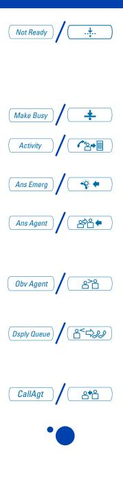
Press the Not Ready Key to put the agent position in a Not Ready state. The Not Ready state takes the agent out of the ACD queue without logging the agent out. The Not Ready state allows the agent to perform and record post call processing duties connected to ACD calls.
