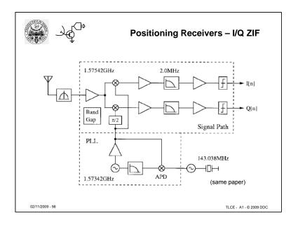
A I/Q structure with direct conversion (ZIF). IF Filters become low-pass.
