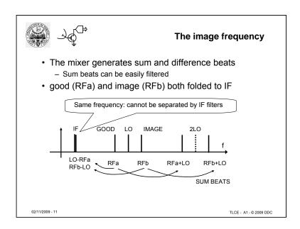
The mixer brings to the same IF frequency two RF signals, RFa and RFb, with frequency respectively:
