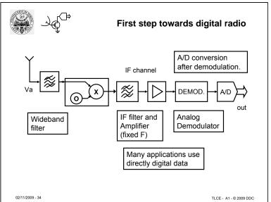
A first choice is to place the ADC at the end of the receiver chain, after the demodulator. On demodulated signal represented by numeric samples, it is possible to apply error correction, encryption or other functions that can be easily implemented on digital signals.
