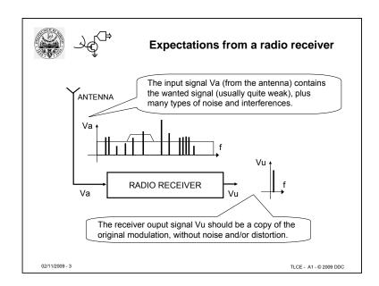
A radio receiver can be seen as a system which converts RF signals (Va in the diagram), collected by an antenna, and extract the information contained in one of the "channels" (e.g. a radio station), converted to a suitable representation (e.g. an electric signal Vu, able to drive earphones or other transducers).
