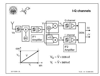
The receiver may use I/Q demodulation, to keep amplitude and phase information.
