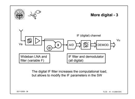
The next step is to place the A/D converter at the input of the IF chain, just after the mixer.
