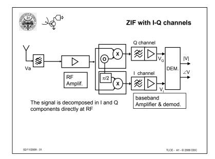
ZIF radio architectures are widely used inside ICs, mainly because lowpass filters are more easy to design and build than band-pass.
