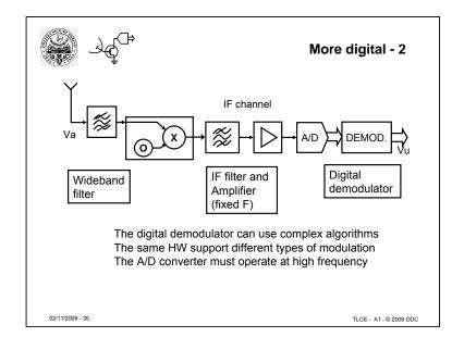
A second choice is to place the A/D converter at the end of the IF chain, between the IF output amplifier and the demodulator.
