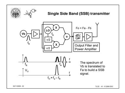
A more interesting application is in SSB transmitters. A standard AM signal includes the carrier and two sidebands; since each sideband carries all information, higher efficiency is achieved by keeping only one of the sidebands. The benefits are
