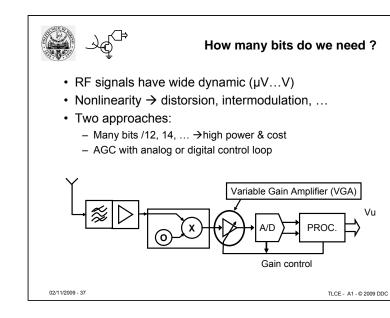
A key parameter in complex digital processing (such as filters) is the resolution (or precision) of the computation (the number of bits). To get a high resolution the ADC must provide a high number of usable bits, over all possible signal values.
