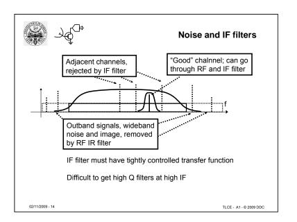
The effect of frequency translation and IF filtering is like placing a narrow band-pass filter (IF bandwidth) on the RF signal. When LO is moved, the effect is the same as a tunable band-pass with a high Q.
