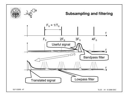
The RF signal must be filtered before the sampling.
