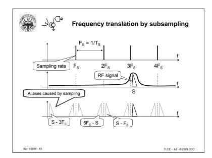
Now the sampled signal has a spectrum just above 3Fs, with a bandwidth Fb. Sampling at Fs rate creates the set of aliases. If the bandwidth Fb is < Fs/2, these aliases are not overlapped.
