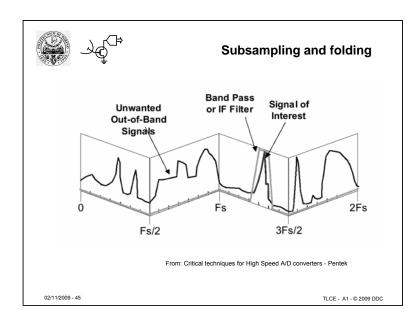
Spectrum folding overlaps several parts of the spectrum; to keep (in each fold) only the useful signal, this must be filtered (pass-band) to eliminate/reduce outband noise and interferers. Here we have the filtering effect: by filtering, so isolating the set of the
