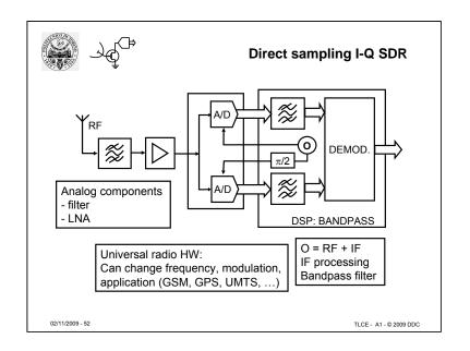
Same principle (all digital processing) with direct sampling. Down conversion carried out by sampling, without mixer. Image cancellation uses I/Q processing Sampling rate is related with RF bandwidth Sampling jitter is related with carrier frequency.
