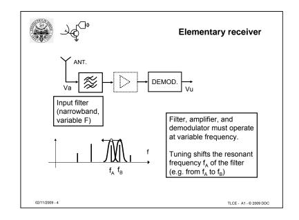
The block diagram shows the most simple architecture for a receiver:
