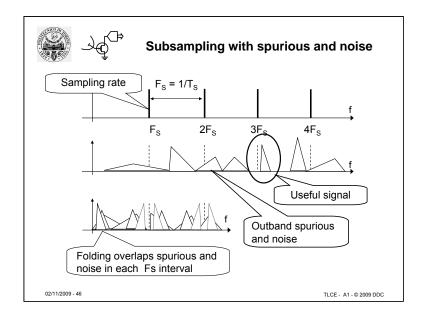
Subsampling unfiltered signals brings to overlapping of various spectrum segments. Outband signals become inband noise, which cannot be isolated later
