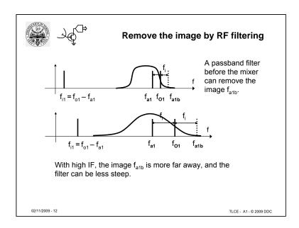
A pass-band filter on RF before the mixer can remove the image. The RF filter bandwidth must cover all the input frequency range of the receiver
