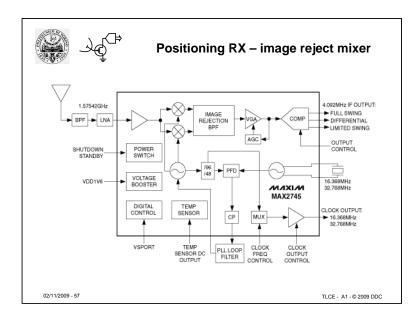
Block diagram of a commercial IC, where it is possible to recognize -I/Q architecture (not a ZIF, since the IF filters are bandpass) -VGA controlled by an AGC circuit -I/Q Local Oscillator
