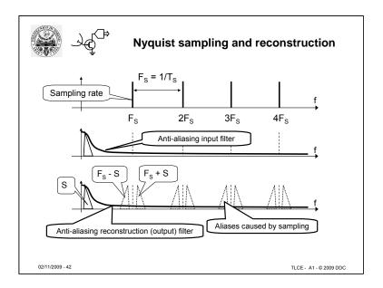
The slide shows the effect of sampling on signal spectrum. Compliance with the Nyquist-Shannon rule (Fs > 2 Fb) guarantees that aliases are not overlapped, and the original signal can be recovered by low-pass filter.
