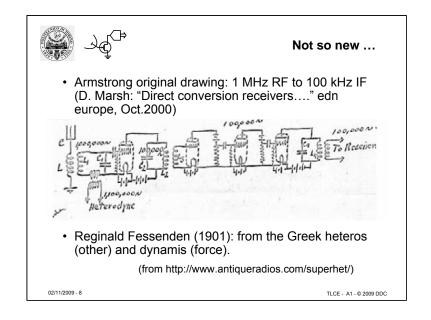
The principle of heterodyne (or use of beats) is well known; the slide shows the schematic diagram of an heterodyne receiver with electronic tubes (triodes).
