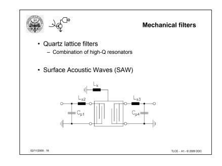
Good band-pass filters are expensive & bulky, and achieving a specified shape can be difficult. Available technologies include
