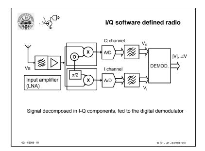
The slide shows a digital I/Q radio system.
