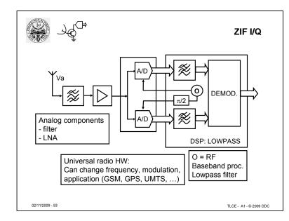
This is the same structure as in previous slide, but here the RF is moved directly to baseband (DC): we get a Zero IF (ZIF) system.
