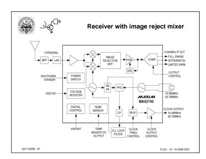
Example of complete radio chain in a commercial IC (GPS receiver). In this diagram we can recognize several elements of an I/Q receiver. -The PLL loop for the LO -The VCO with direct sin/cos outputs -The image rejection unit
