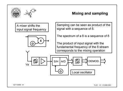
Sampling corresponds to multiplying a signal by a sequence of pulses, spaced by the sampling interval Ts. The spectrum of a sequence of deltas is a sequence of delta (in the frequency domain), spaced by the sampling rate Fs = 1/Ts.
