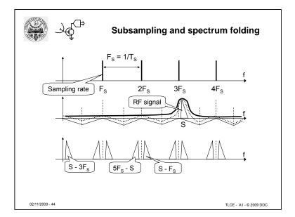
The generation of aliases can be represented with a folding process. The spectrum is drawn on a strip of paper, which is folded at Fs/2, Fs, and multiples of Fs/2. The signals present in each fold are copied (by the sampling) to all other segments.
