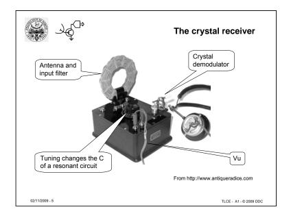
This is an example of radio system based on the previous architecture: a "Galena" receiver.
