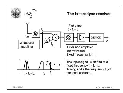
In this diagram the RF signal from the antenna is filtered (wideband input filter) to remove outband noise, then multiplied by the Local Oscillator signal Fo; this causes a shift in the frequency domain to the sum and difference beat positions.
