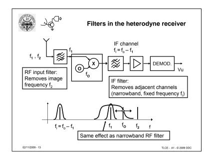
The RF input filter (band-pass, wide) removes noise and interferers outside the band used by all received channels; all channels are still present at mixer input.
