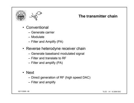
Up to now we have seen radio architectures for radio receivers; transmitters can use the same approaches, that is:
