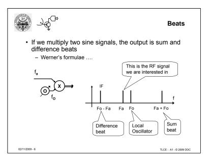
The slide is a refresh on what happens when we multiply two sine signals, with frequencies respectively fa and fo.
