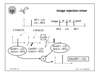
Besides generating SSB signals, I/Q signal processing can be used to cancel the image signals in a receivers.
