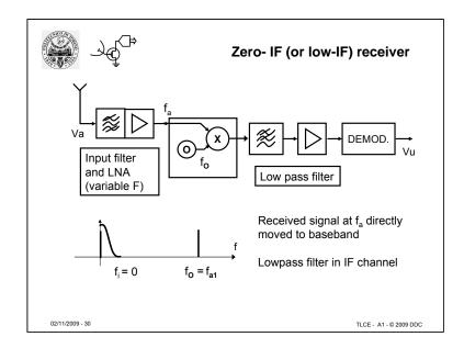
The heterodyne moves the signal spectrum to IF, usually lower than RF; Zero-IF receivers apply the same principle, but move the signal spectrum to DC (LO has the same frequency as the desired channel). This is called Zero IF (ZIF).
