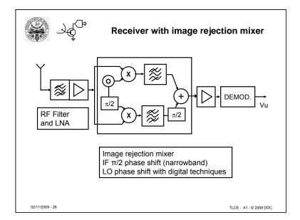
The image rejection I/Q mixer is here used in the receiver chain, after RF filter and LNA.
