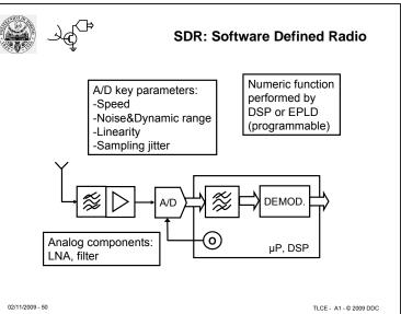
The block diagram in the slide shows a radio system where all functions (besides RF filter and amplifier) are carried out by digital units, after the ADC.
