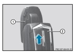
► Push telephone module ② into fixture ① until it engages audibly.
