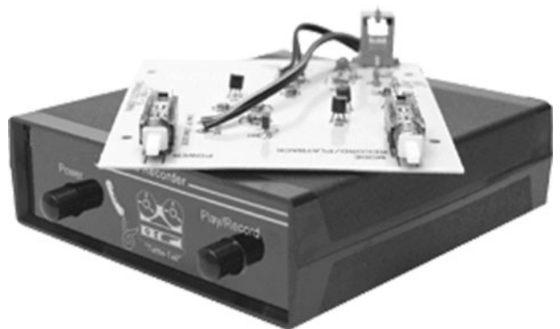
Figure 9-1 Automatic telephone recording switch
