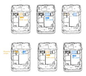
To insert a Nano SIM or microSD card, push the Nano SIM or microSD card into the corresponding card slot with the gold-connectors facing down. To remove the Nano SIM or microSD card, push down on the plastic clip and pull the Nano SIM or microSD card out.
