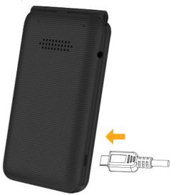
Insert the micro USB cable into the phone's charging port and plug the charger into an electrical outlet.
