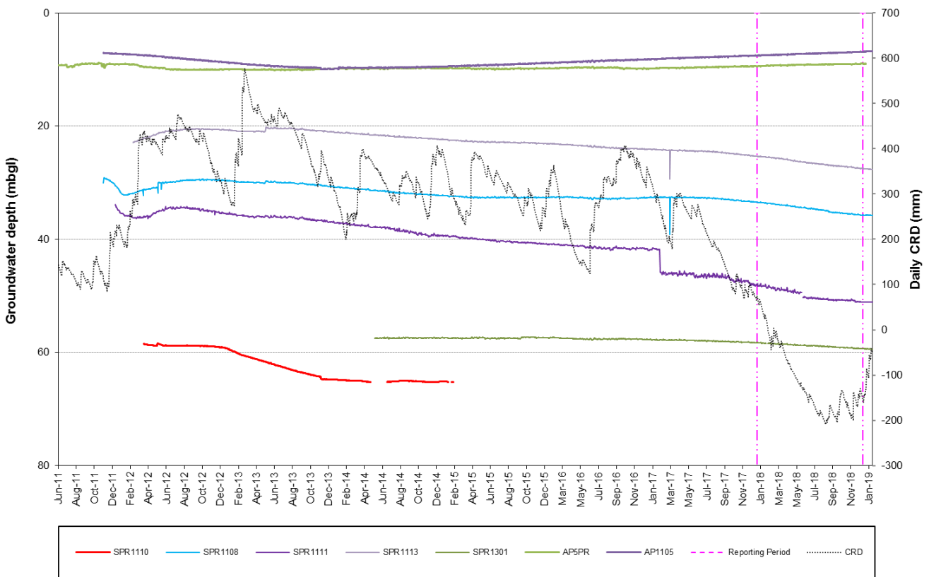
Figure 14 SPR1110 and Reference Ridge Piezometer Hydrograph - 2011 to 2018
