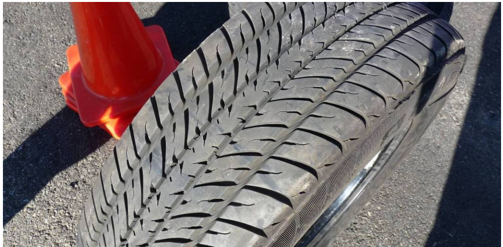
Figure 5.1. A Goodyear Aquatred tire.
