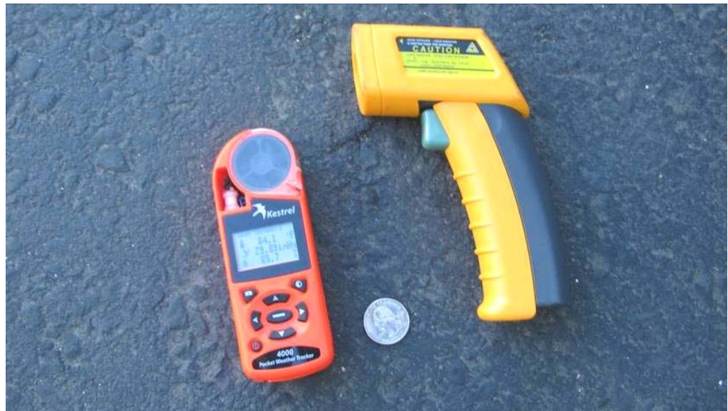
Figure 3.3. Pocket weather station and Fluke thermal infrared gun used to measure respectively air and pavement temperature.
