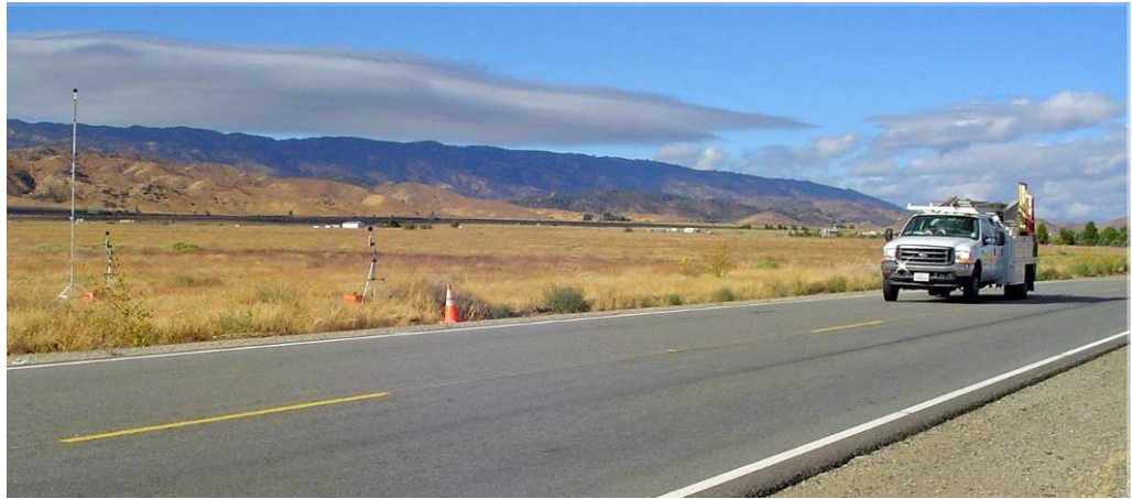
Figure 1.11. The roadside SPB noise measurement setup at LA138 test road in the Mojave Desert (Photo Judith Rochat, VOLPE).
