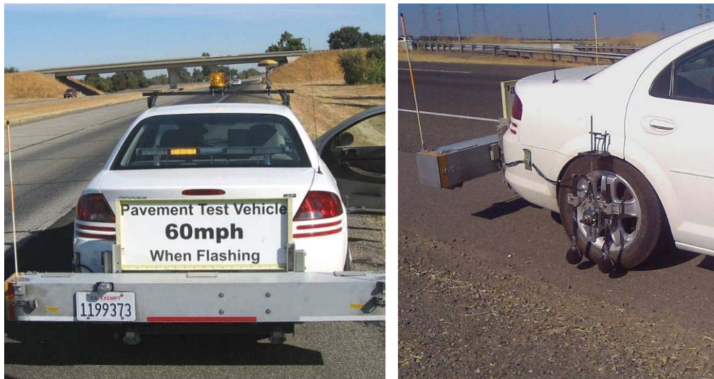
Figure 3.1. The UCPRC OBSI measurement vehicle.
