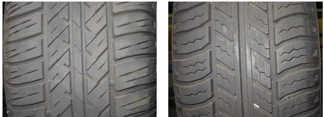
Figure 1.14. The two Michelin summer tires used in the French experiment. The “noisy” Tire A to the left and “low noise” Tire B to the right (photo Fabienne Anfosso-Lédée, LCPC).
