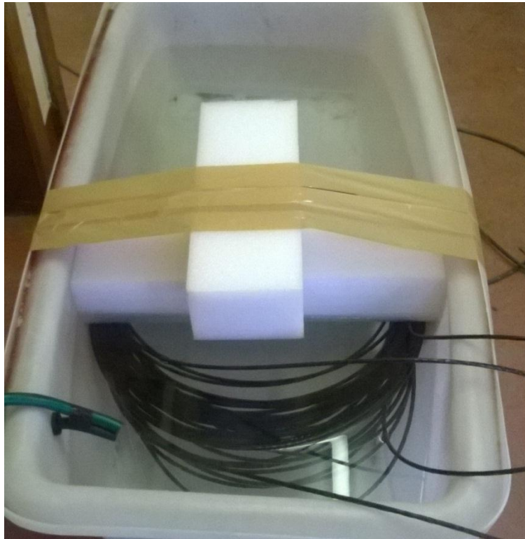
Figure 19: Water bath technique used for DTS calibration and maximum temperature alarm test
