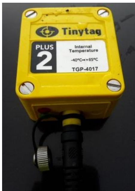
Figure 21: Temperature sensor and data logger, Tinytag
