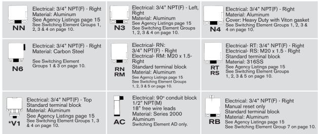
Hazardous Locations - Hermetically Sealed Switching Element NEMA 4, 4X, 7, 9, IP66
