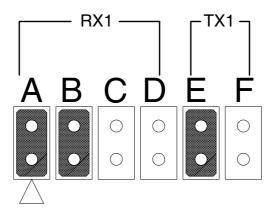
Figure 2.20 Active Mode Jumper Setting
