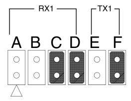
Figure 2.21 Passive Mode Jumper Setting
