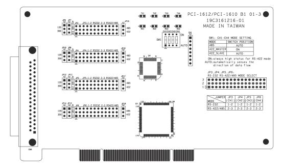
Figure 2.6 PCI-1610A/B, PCI-1612A/B Silk Screen
