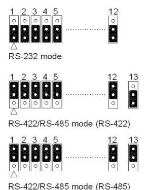
Figure 2.15 PCI-1612 Series RS-232/422/485 Selection
