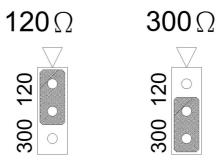
Figure 2.22 Resistor Selection (for PCI-1612/1622 series)
