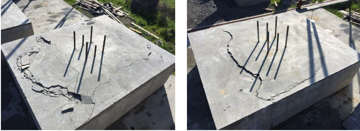
Figure 5 – Overhead view of breakout surface for (a) 12-inch embedment and (b) 18-inch embedment
