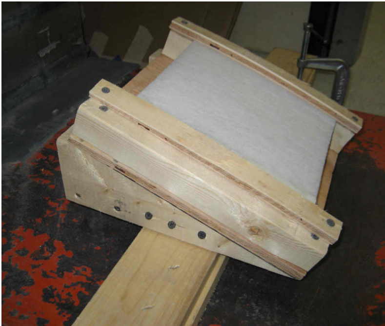
Drum vibrator with aerogel blanket
