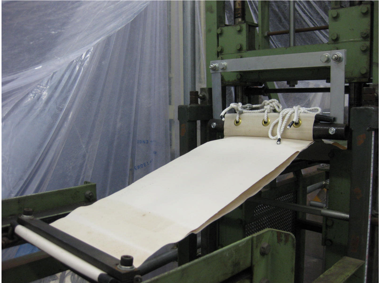
Snap test apparatus to test mechanical fastening of aerogel blanket
