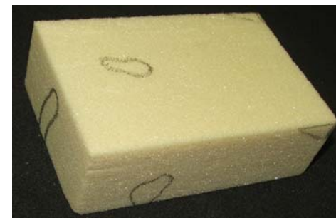
Coupon with defects marked after x-ray inspection
