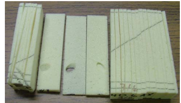
Coupon with defects after final dissection
