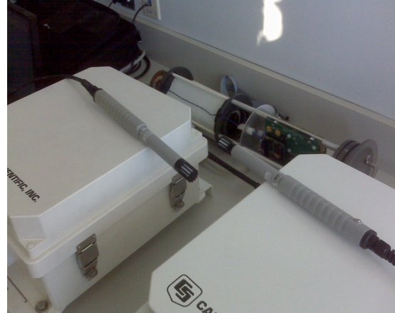
Fig 3. Temp./RH probes during bench top testing on 17 Oct 2008
