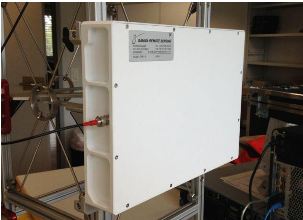
Figure 10 : RF Assembly mounted on the antenna tower. On the left side is the BNC GPS antenna connector.
