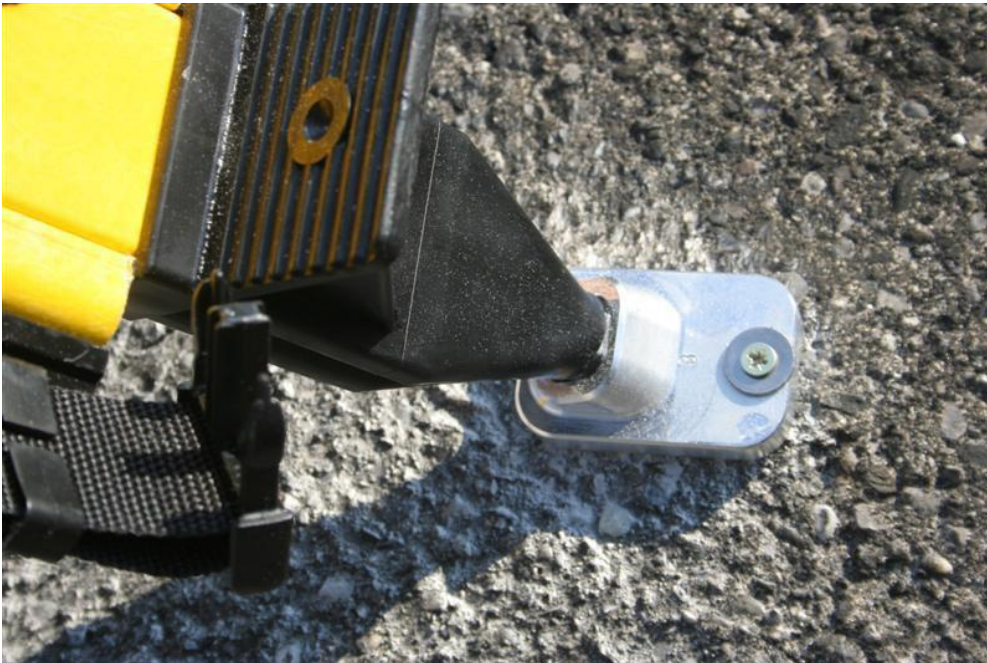
Figure 16: Tripod mounting adapter for screw anchor mounting.
