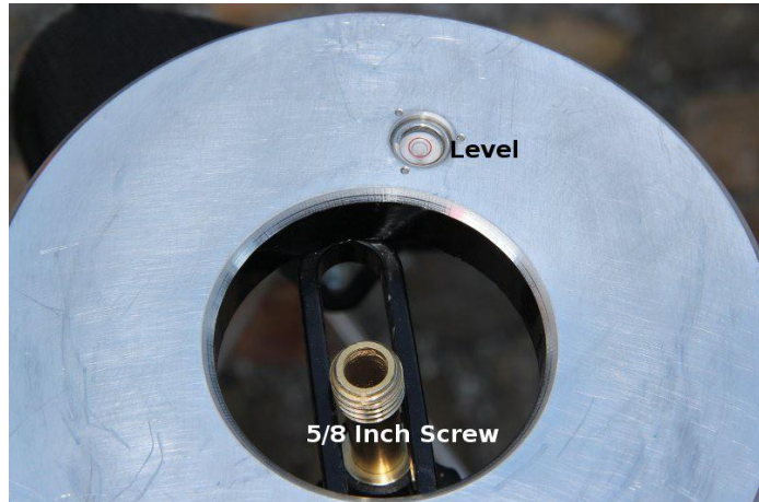
Figure 5: Interface Plate of the Tripod with level and 5/8" hollow screw. The small level is used to ensure that the tripod is level after the feet are locked.
