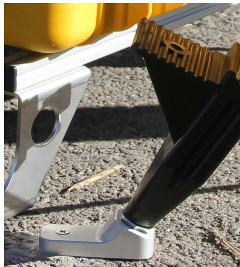
Figure 3: Tripod feet that permit screwing down the legs at fixed positions
