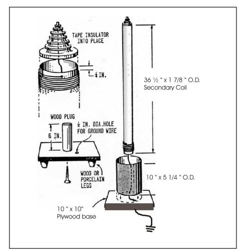
Figure 1-20. Base for coil is made from a 3/4" plywood base
