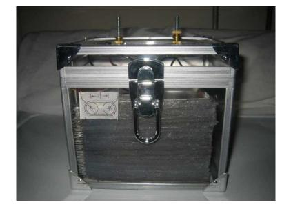
A multi-stack HV Capacitor using clear 4 mil mylar.
