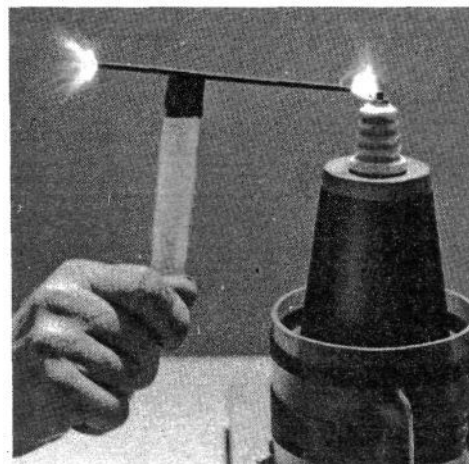
Sample experiments include (top) lighting a fluorescent tube by simply moving it into the high-frequency current field surrounding the coil; (center) lighting a 115-volt light bulb without plugging it into a power line—by means of energy radiated to a sheet-metal plate; (bottom) passing the current from the coil's own brush discharge through a metal rod taped on a plastic strip to form a duplicate brush at the other end
