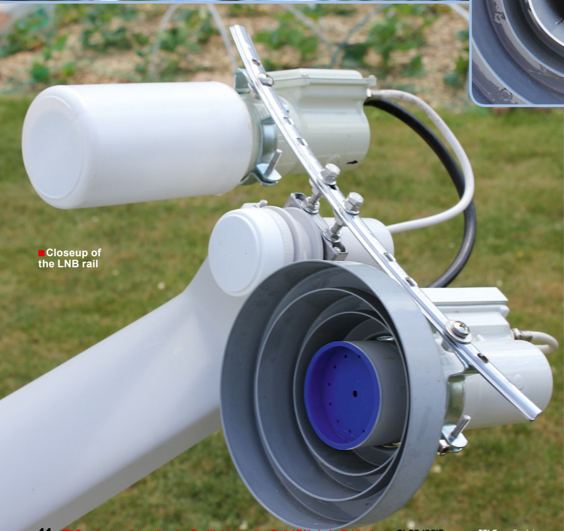
■ A look inside the feed reveals the polarization probe
