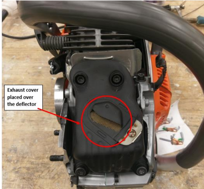
Figure 11 Image of Husqvarna 550 XPG Chainsaw Muffler
