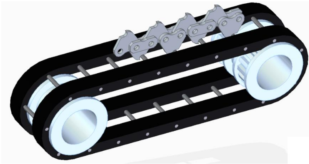
Figure 6 CAD of Modified Chain on Timing Belt
