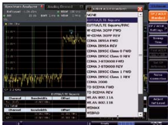
ACP measurement: a wealth of predefined standards included to simplify making settings.
