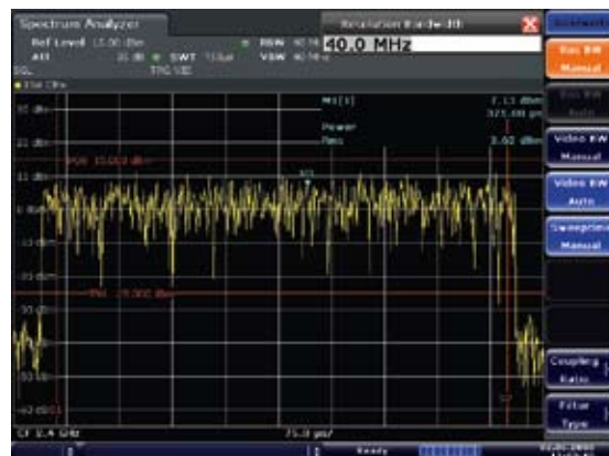
Measurement of the power of a wideband WLAN signal using the time domain power function.
