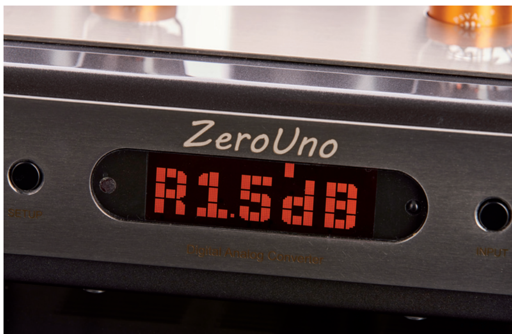
The display of the ZeroUno DAC showing the "Balance" control at plus 1.5 dB for the right channel
