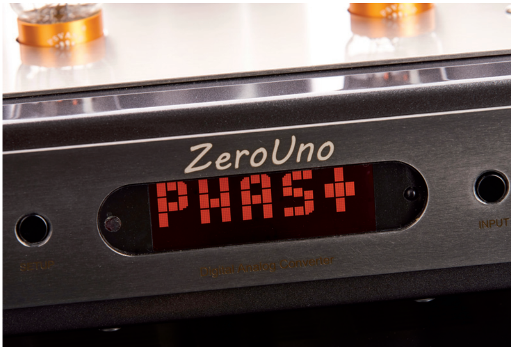
The display of the ZeroUno DAC showing the phase in absolute polarity (+)
