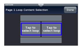
3. Press on each content block above selecting **Temperature** for the left and **Humidity** for the right (Humidity is only applicable on Temperature/Humidity chambers). Pressing the **Temperature** or **Humidity** area in the **Loop Content Selection** screen will bring up the ability to select the color.
