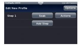
Each new step will automatically be a copy of the previous step. You can then edit the parameters of the new step to suit your profile.
