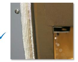
Figure 11: Chamber Gasket Aligned
